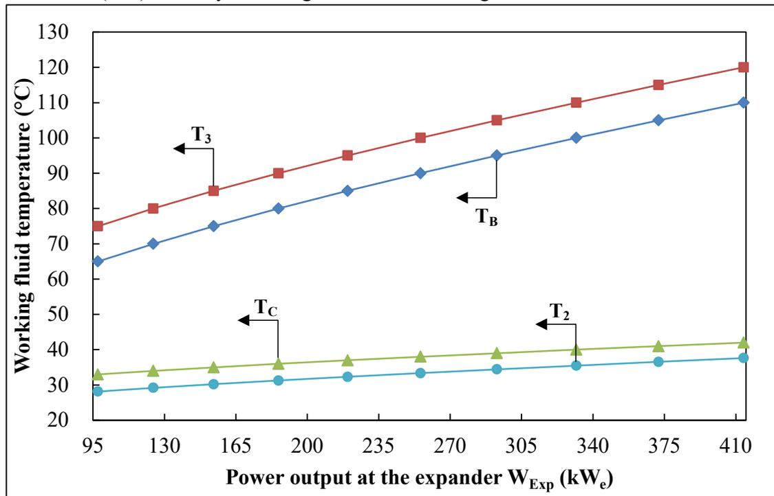
**Fig. 4.** Working fluid temperature in the ORC system.
