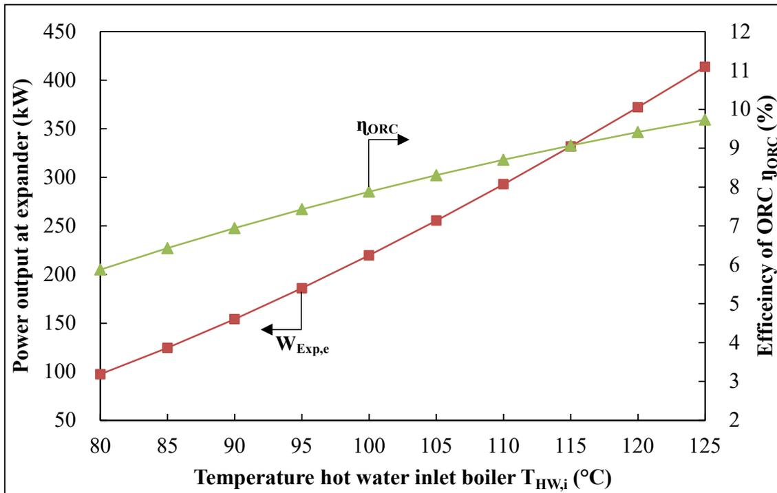
Fig. 6. Energy efficiency of the ORC system.
